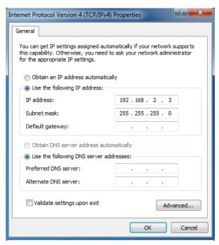
IP Address of the computer should be at the same network. For example – 192.168.2.3. Into the browser you should type <a href="http://192.168.2.2">http://192.168.2.2</a>. If network settings are correct the login page will appear.
